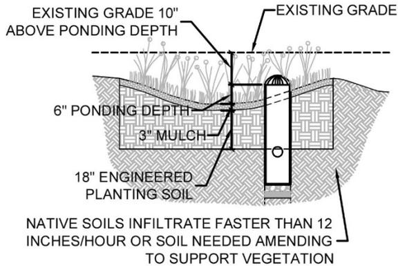
**Infiltration testing depth = 10" (elevation difference) + 6" (ponding depth) + 3" (mulch) + 18" imported soil = 37 inches below existing grade**
