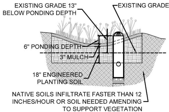
**Infiltration testing depth = -13" (elevation difference) + 6" (ponding depth) + 3" (mulch) + 18" imported soil = 14 inches below existing grade**
