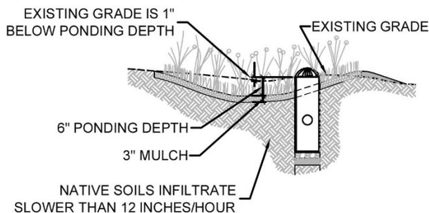
**Infiltration testing depth = -1" (elevation difference) + 6" (ponding depth) + 3" (mulch) = 8 inches below existing grade**
