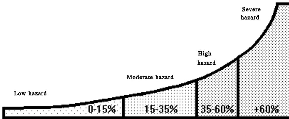
The percentage of slope is found by dividing the vertical rise by the horizontal run of a specific area of the slope.
