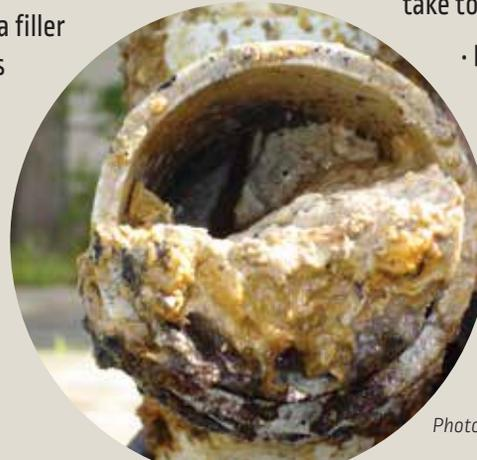
*Photo of a pipe filled with FOG.*
